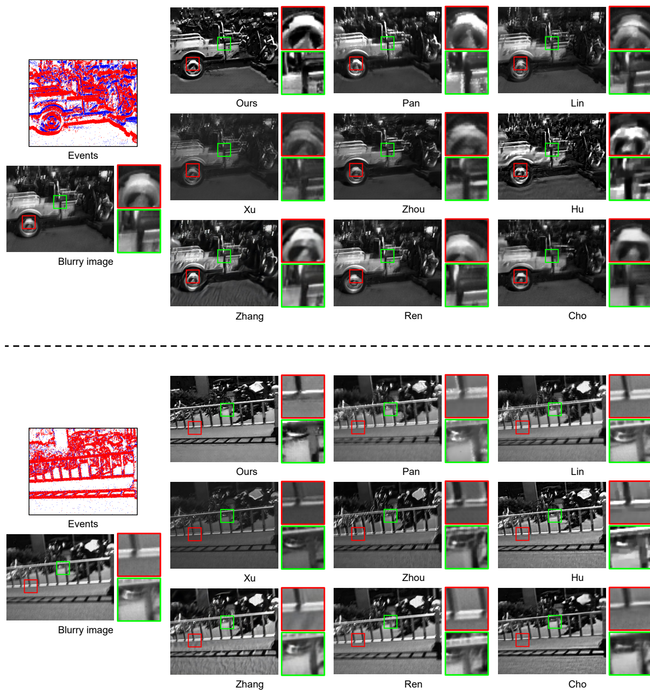
Fig. 12 Additional qualitative comparisons on real data captured by an event camera among our method, four event-based deblurring methods (Pan et al, 2019; Lin et al, 2020; Xu et al, 2021; Zhou et al, 2021), and four image-based deblurring methods (Hu et al, 2018; Zhang et al, 2019; Ren et al, 2020; Cho et al, 2021) (part 3).
